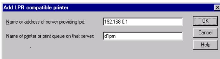
6. Type in the IP address or host name of the M202, M202Plus, M205, M305 and M307 in the first field.
