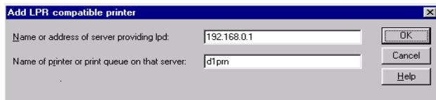
The first field specifies the IP address for the M202, M202Plus, M205, M305 and M307 and the second field must be filled in with an existing destination on the print server (e.g. d1prn). Otherwise, the M202, M202Plus, M205, M305 and M307 won't accept this as a valid network printer.
